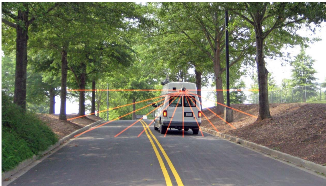
Figure 15 Instrumented Van with 360-degree rotating laser measurement device
